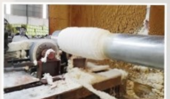
Automated Spray Pre-Insulated Pipe
